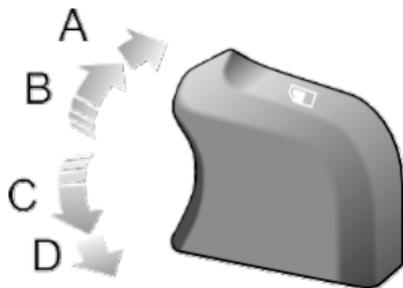
Press the window control switch (as shown in Figures 2~5) down to the 1st position (Position C) to lower the window and pull the switch up to the 1st position (Position B) to raise the window. The window will stop moving as soon as the switch is released.
